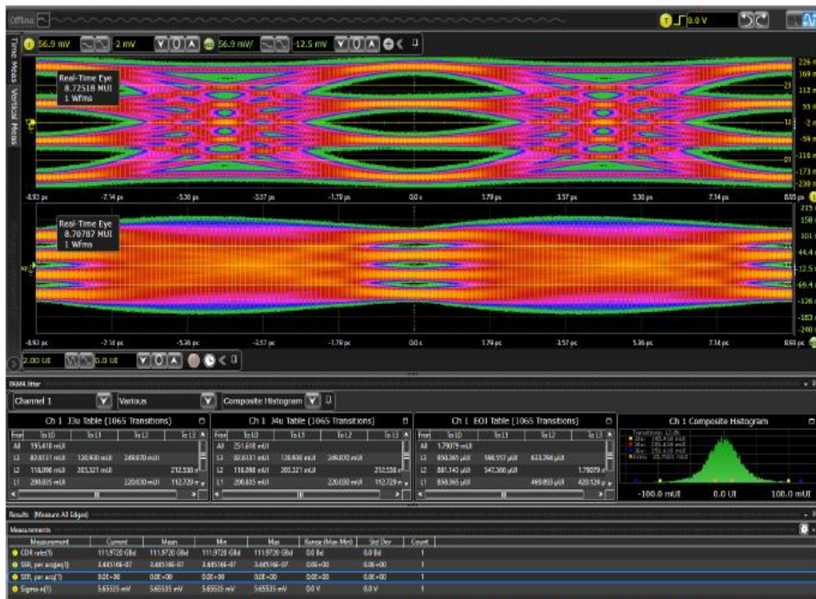
Figure 13 Real-Time instrument measurement of a 112 GBd PAM4 precision stimulus system incident to the illustrated packages
