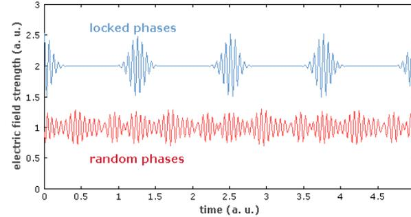
**Passive mode-locked** uses a saturable absorber incorporated into the laser cavity
